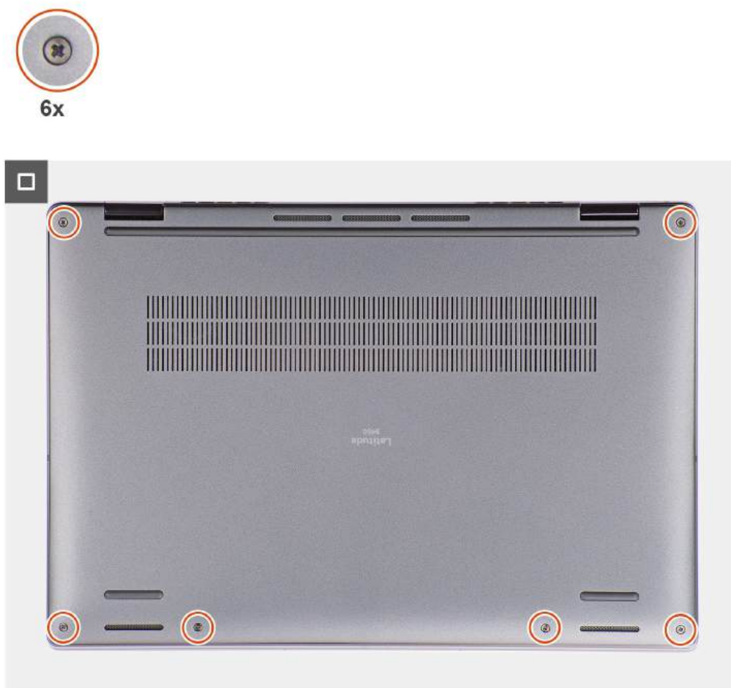
Figure 19. Installing the base cover
