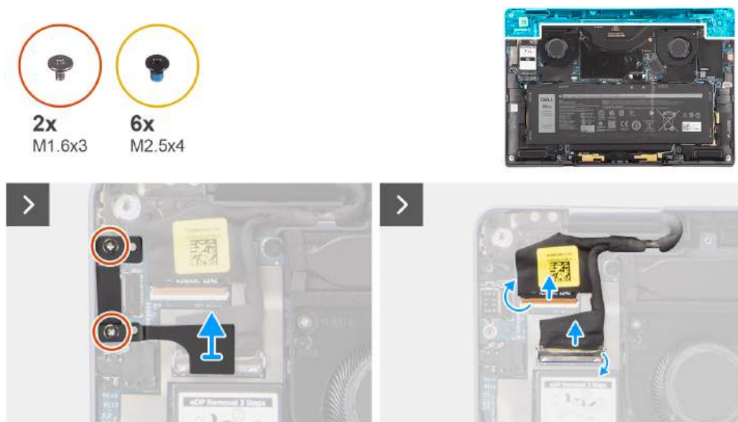
Figure 47. Removing the display assembly
