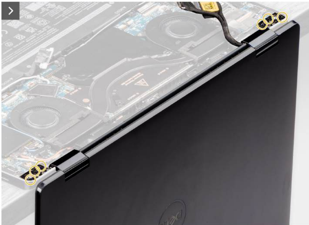
Figure 49. Removing the display assembly
