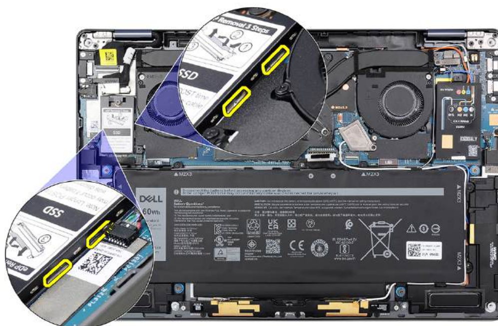
Figure 25. Solid state drive shielding cover
