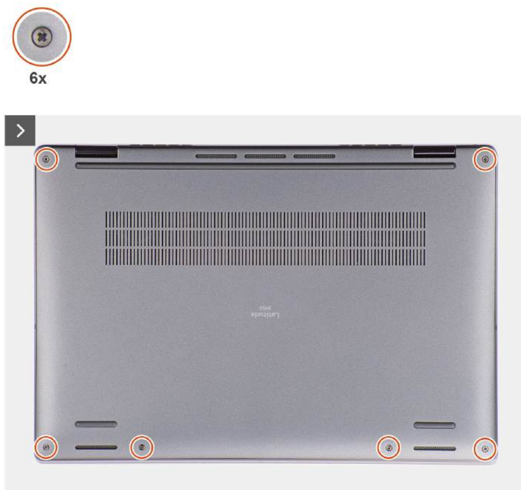
Figure 15. Base cover removal
