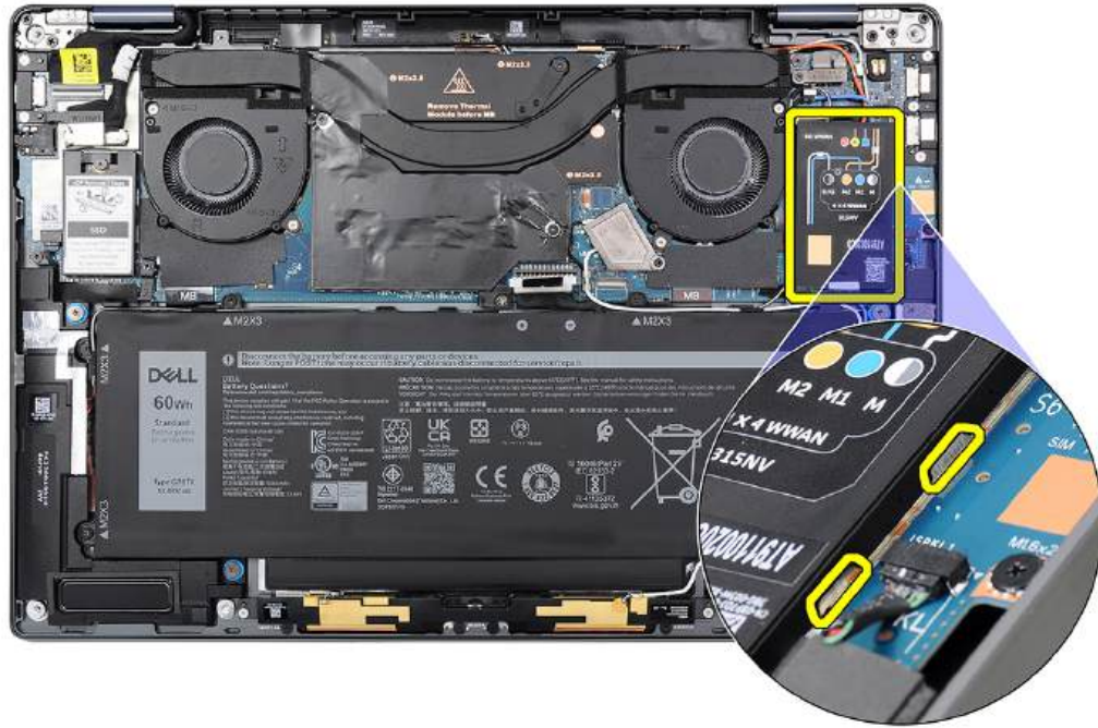
Figure 28. WWAN-card shielding cover
