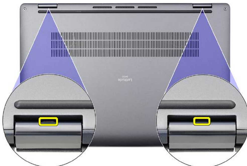
Figure 17. Base cover pry points
