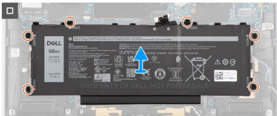
Figure 33. Removing the battery
