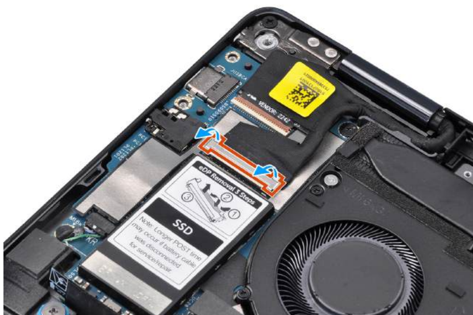
Figure 48. Disconnecting the display cable
