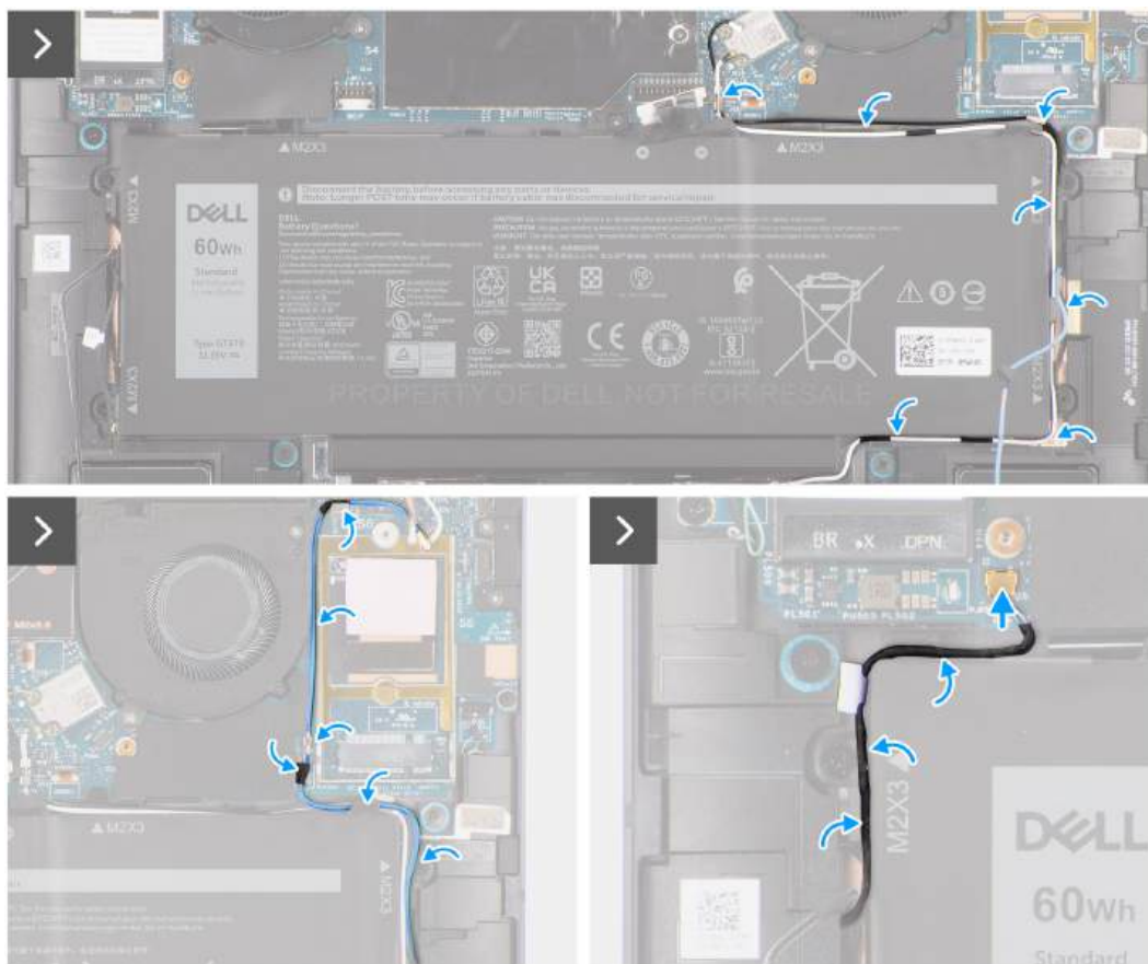
Figure 35. Installing the battery
