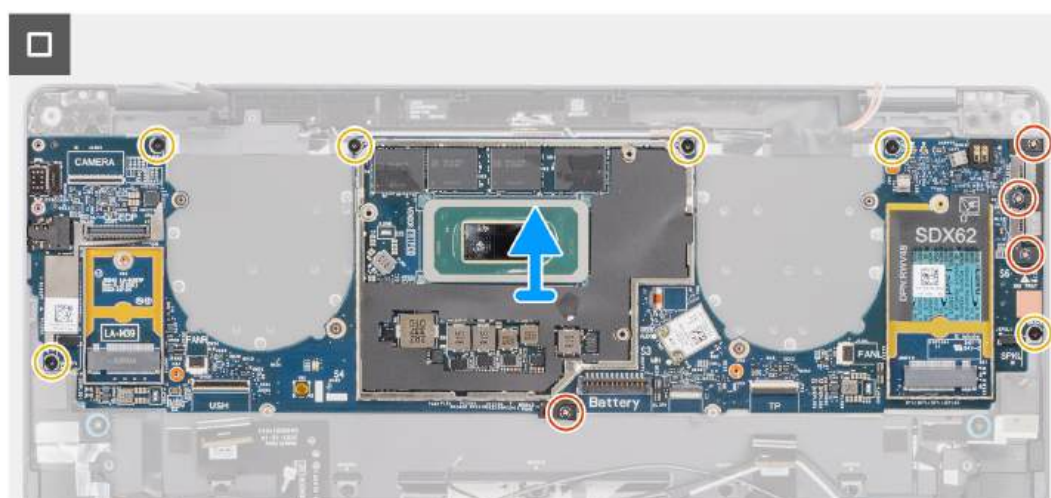
Figure 55. Removing the system board
