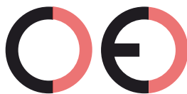
False CE Mark (too far)
